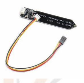
This capacitive soil moisture sensor V2.0 measures soil moisture levels by capacitive sensing rather than resistive sensing like other sensors on the market. It is made of corrosion-resistant material which gives it excellent service life. Insert it into the soil around your plants and impress your friends with real-time soil moisture data!
